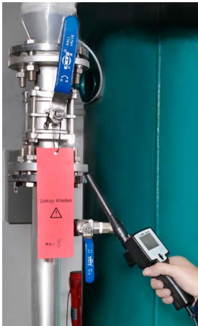
The new CS 530 ultrasonic leak detector is designed to allow the user to identify leaks quickly
