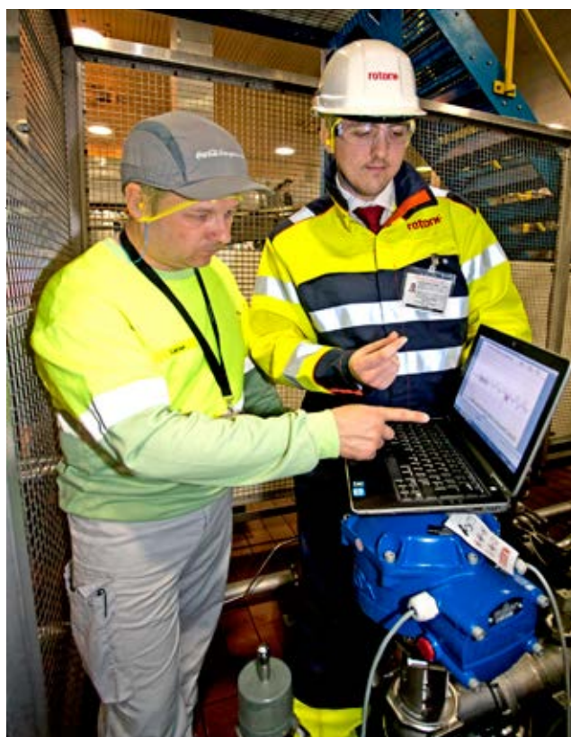
A Rotork engineer demonstrates the improved control valve performance illustrated by the Rotork CVA actuator's datalogger.
