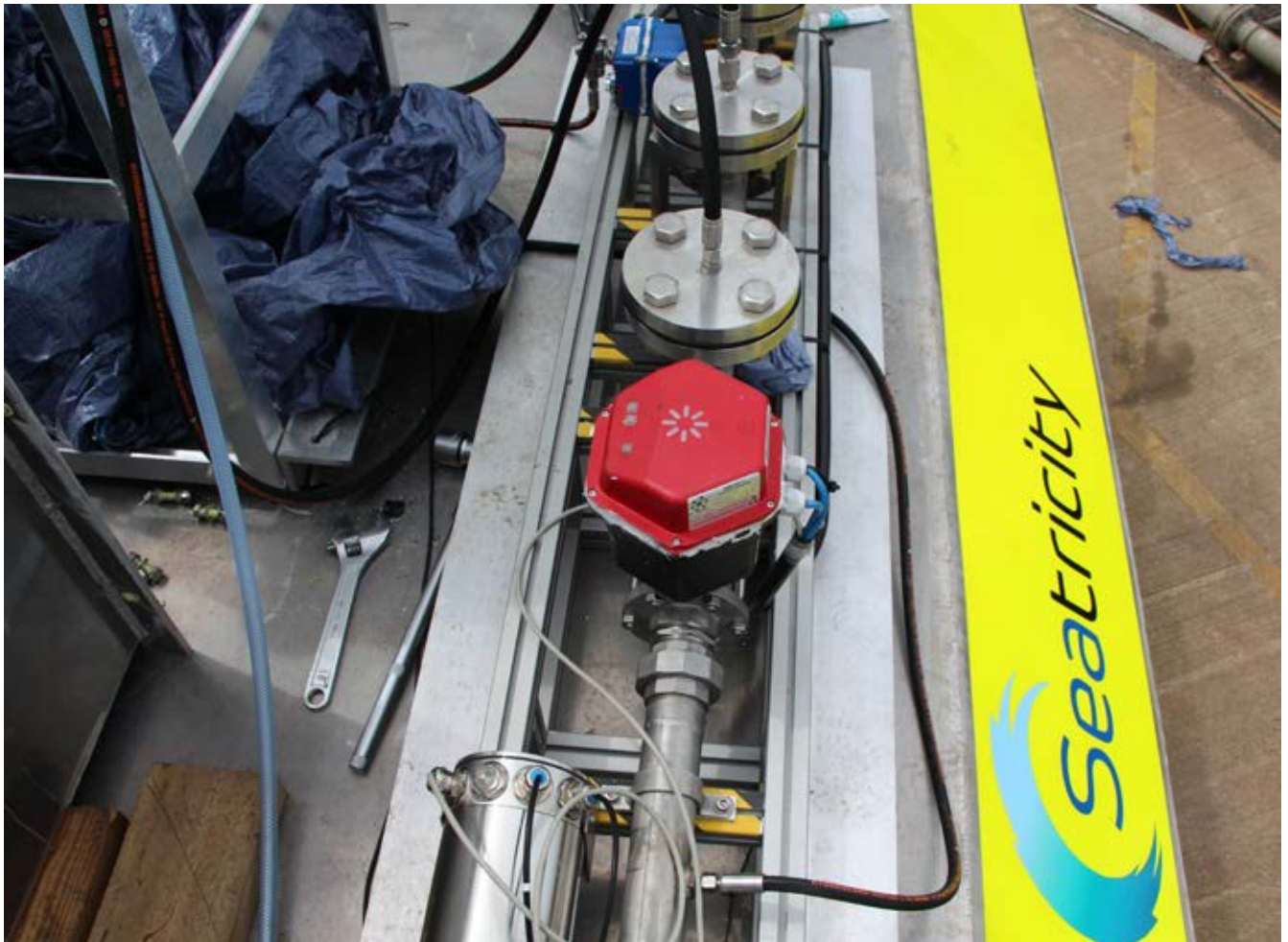
The Mars valve and SACO SmartAct®-1 actuator low-energy valve solution will use solar power to correlate wave movement with power generated on the Oceanus 2 wave device
