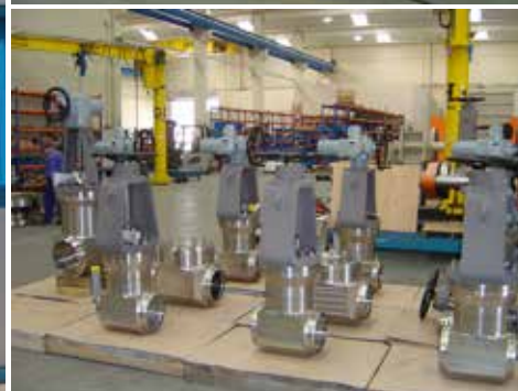
Left: José Manuel Garcia Monclus, MD of Ringo Valvulas and Roy Wood MD of DVL shake hands on their partnership Top Right: A 36" 1500 psi valve from Ringo Bottom Right: Nuclear forged gate and check valves
