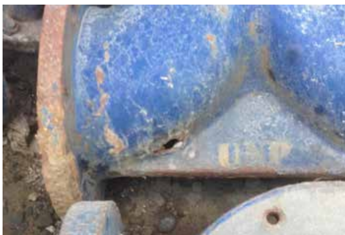
CORROSION: Weir type PTFE lined diaphragm valve on a Sulphuric Acid duty
