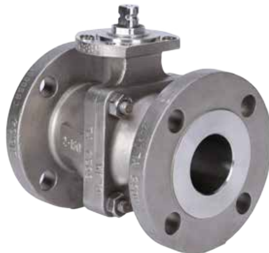
Image: Self-relieving seats relieve excess pressure to protect the integrity of the valve while maintaining bi-directional operation
