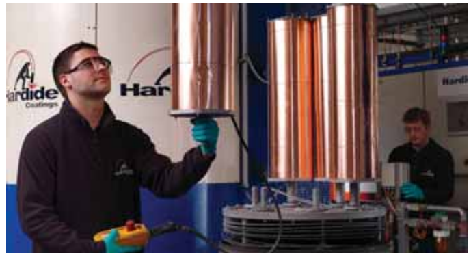
Hardide coating reactor being loaded with components
