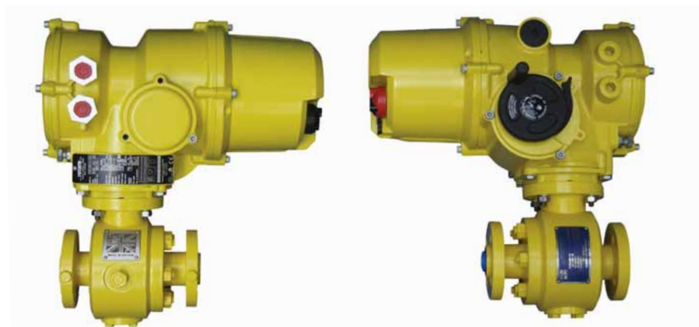
Looking to alternative markets... 1" ASME 600 'Phase' Ball Valves (316 Ti + Hardide coating) complete with Rotork IQT actuators for a nuclear application (Heap & Partners)
