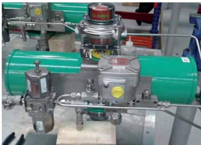
3" butterfly valve with pneumatic spring return actuator with all controls
