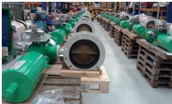
12" butterfly valve with pneumatic spring return actuator
