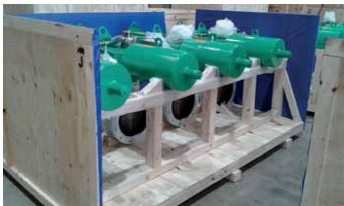
12" actuated valves housed in the packing cases to avoid damage during transit
